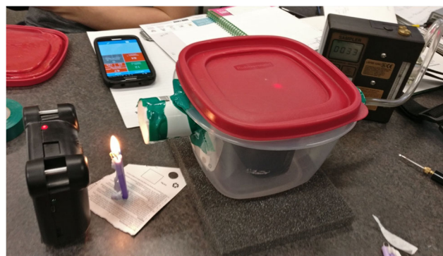
Fig. 2 Student-designed apparatus for investigation of the PM_{2.5} filtration efficiency of disposable dust filtration masks
