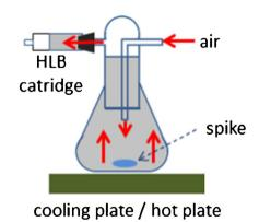
Fig. 2 Set-up for the spiking of the analytes by volatilization
