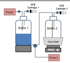
Fig. 3 Set-up of the pseudo-partitioning experiment
