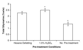
Fig. 3 Comparison of silymarin yield in milk thistle seeds after three different pre-treatment methods. *Asterisk* signifies significance (p < 0.05) from the hexane defatting pretreatment condition
