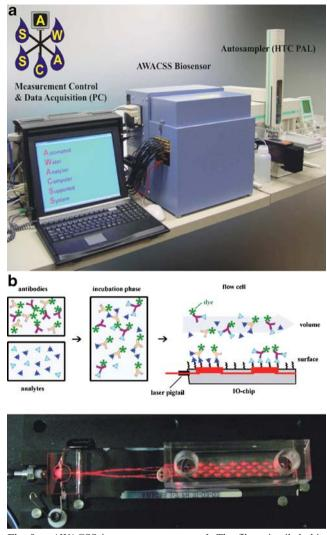
**Fig. 9** a AWACSS immunosensor set-up. **b** The fibre-pigtailed chip with 32 evanescent field-sensing regions (Reprinted in part from Ref. [164] with permission from Elsevier)
