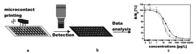
Fig. 1 Schematic diagram of production a, imaging b, and data analysis c for a quantitative analytical microarray
