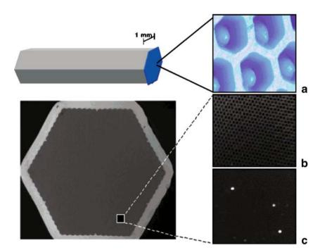
Fig. 14 Fibre optic DNA microarray platform (Reprinted with permission from Ref. [188]; Copyright 2003 American Chemical Society)
