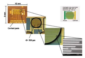
Fig. 7 IDA-electrode structure of an electrochemical microarray (Reprinted in part with permission from Ref. [127]; Copyright 2006 American Chemical Society)
