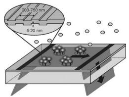
Fig. 6 Evanescent field generation for microarrays using diffractive relief gratings (Reprinted from Ref. [155] with permission from Elsevier)
