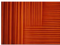
Fig. 4. Experimental picture of a two-variant microstructure in a Cu–Al–Ni alloy, by courtesy of R.D. James and C. Chu
