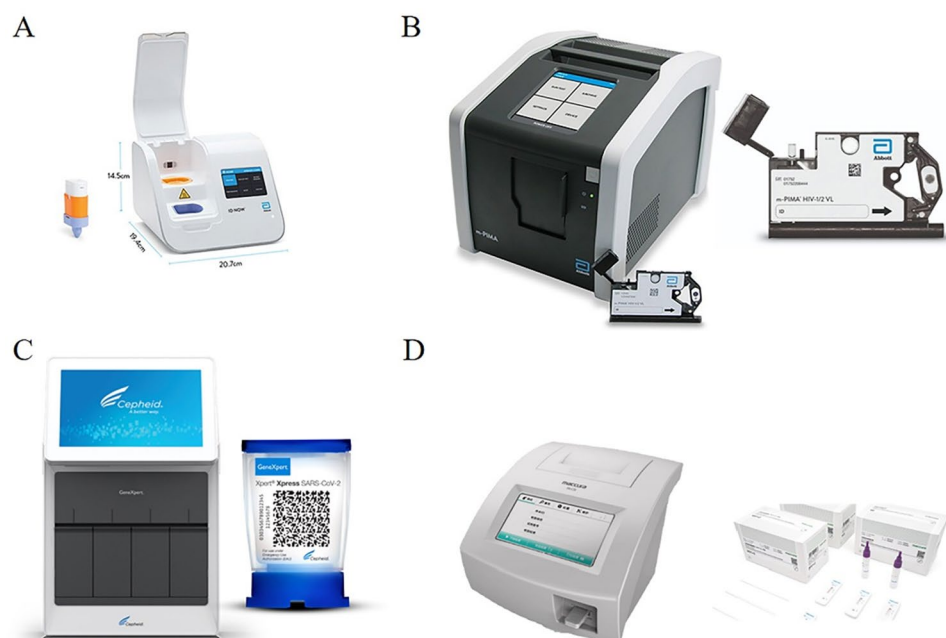
Fig. 14 Systems and tools for POC viral diagnosis are available today. A ID NOW influenza A & B 2 system ( https://www.globalpointofcare.abbott/en/product-details/id-now-influenza-ab-2.html ). B The m-PIMA analyzer and m-the PIMA HIV-1/2 test cartridge ( https://www.globalpointofcare.abbott/en/product-details/m-pima-analyser.html ). C The GeneXpert System and Xpert Xpress SARS-CoV-2® ( https://www.cepheid.com/en-US/systems/GeneXpert-Family-of-Systems/GeneXpert-System ). D R01 fluorescence immunoassay analyzer and Rapid test strip ( https://www.maccora.com/en/product/uwQA2OQdXAE.html )
