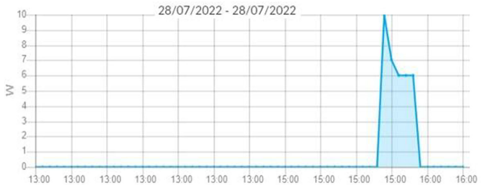
Fig. 25 Conventional PV system laboratory tests: battery power values
