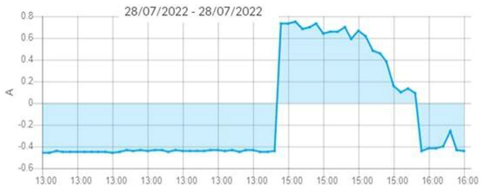
Fig. 24 Conventional PV system laboratory tests: battery current values
