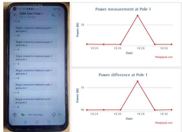
Fig. 19 SMS notification for pole grid 1 (illegal connection identified) and cloud storage results
