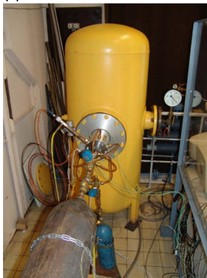
Fig. 4 View of experimental test stand with yellow dump chamber (a) and one of many tested detonation chambers (b)
