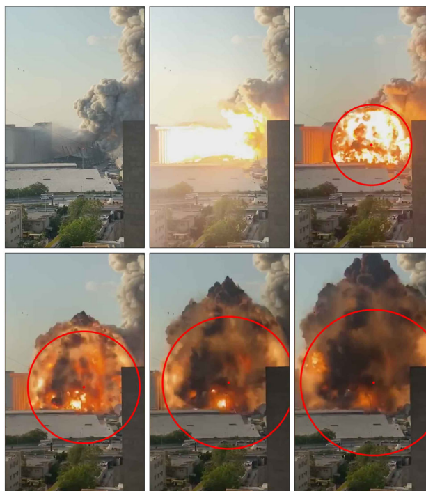
Fig. 12 Video V3 taken from a distance of 666 m from the explosion. Six frames separated by 33.33 ms. The fireball fits are shown as red circles
