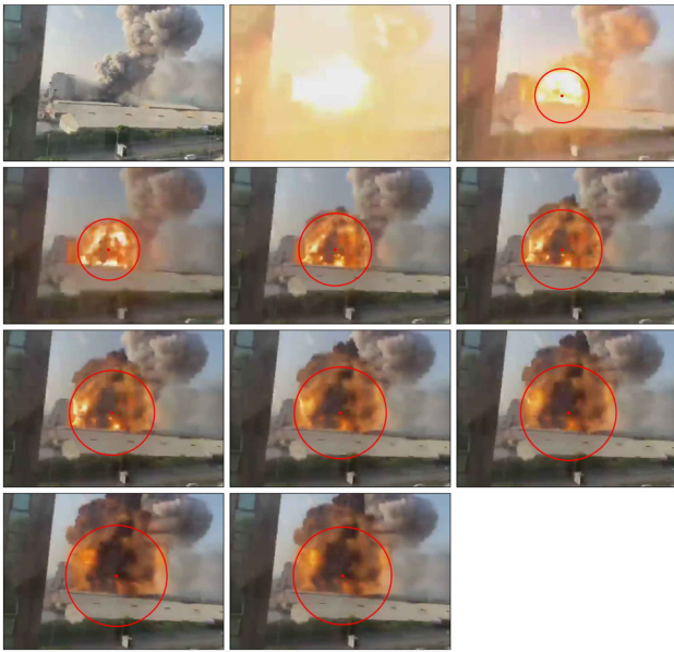
Fig. 13 Video V4 at a distance of 550 m. The fireball fits are shown in red circles
