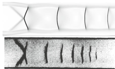
Fig. 4 Numerical schlieren obtained from the reference case using grid A3 (top) and Carroll's [11] experimental schlieren (bottom)
