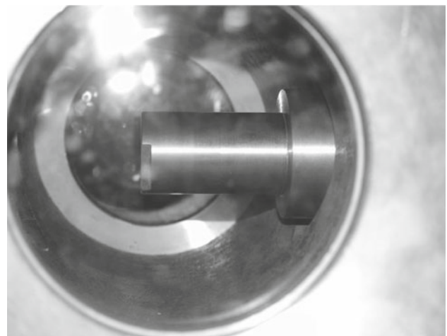
Fig. 4 View of the extension tube inside the visualization chamber
