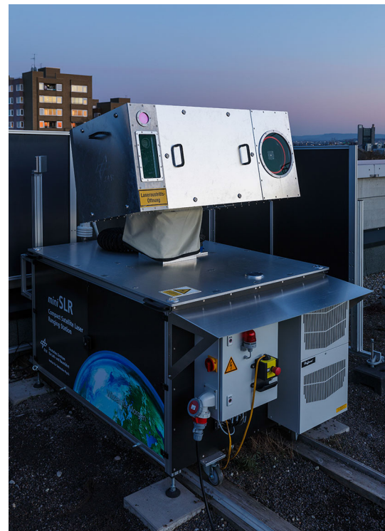
Fig. 1 The miniSLR prototype on the roof of the DLR institute building. The enclosure in the bottom contains most of the electronics and IT. The top compartments house the receive and transmit telescopes, the laser head, cameras, detectors and beam control optics
