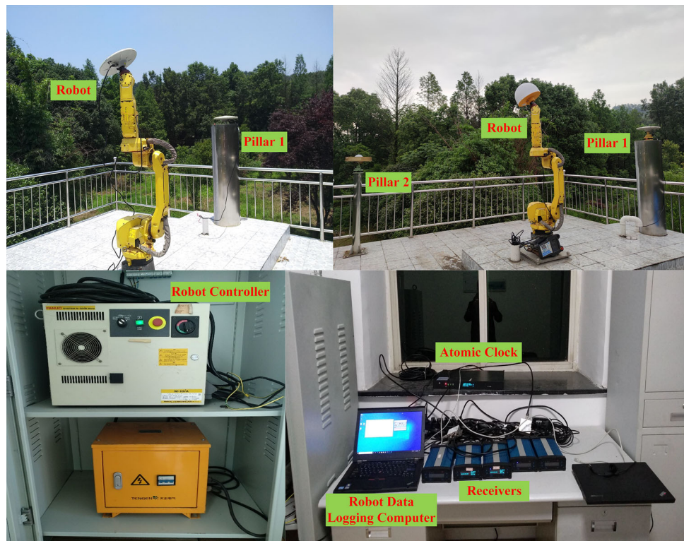
Fig. 2 Field antenna calibration system at Wuhan University. The system is built on a rooftop and includes a six-axis robot, a controller, an atomic clock, receivers and other auxiliary equipment
