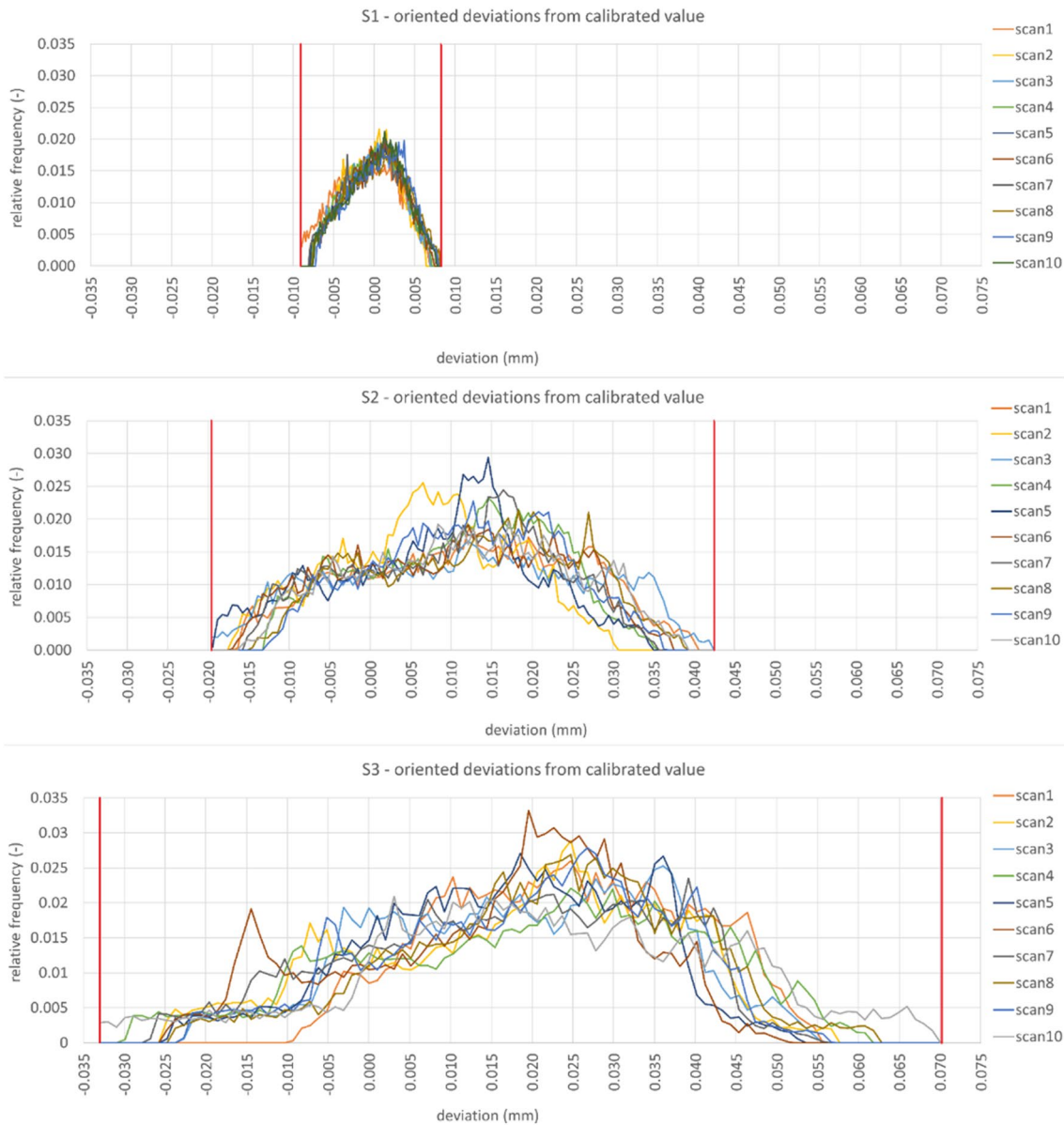
Fig. 7 Oriented deviations from calibrated value for scanners S1, S2 and S3
