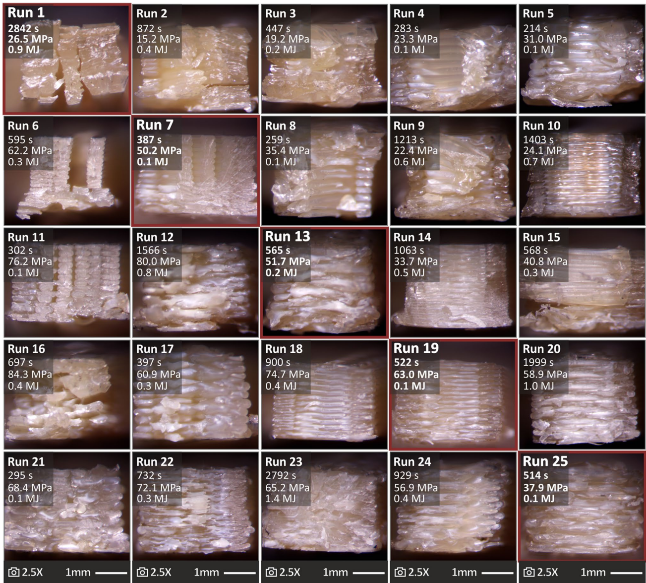
Fig. 6 Stereoscope images from the specimen's fracture surface of the 25 runs (one randomly selected out of the five of each run). The printing time, tensile strength, and energy are also presented in every case
