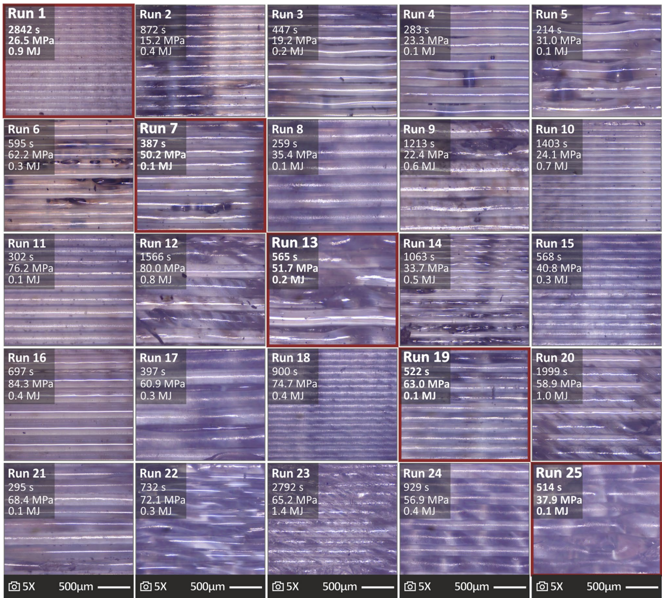
Fig. 5 Microscope images of the side surface of specimens for 25 runs. The 3D printing time, tensile strength, and energy for each sample are also presented
