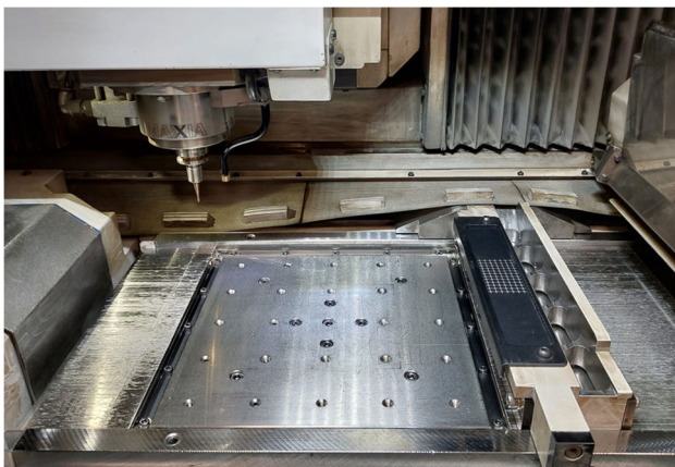
Fig. 2 Hybrid additive manufacturing unit, depicting the recoater, build plate, and the integrated high-speed milling spindle
