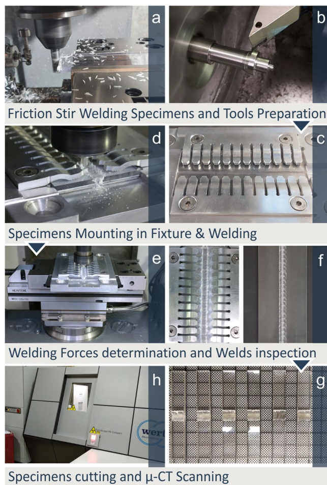
Fig. 1 On the right side, the steps of the experimental procedure are depicted. On the left side, images from the experimental procedure are illustrated a PC sheets preprocessing, b weld tools fabrication in
