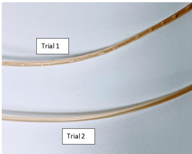
Fig. 2 Filaments cooled using water bath (trial 1) and air curtain (trial 2)
