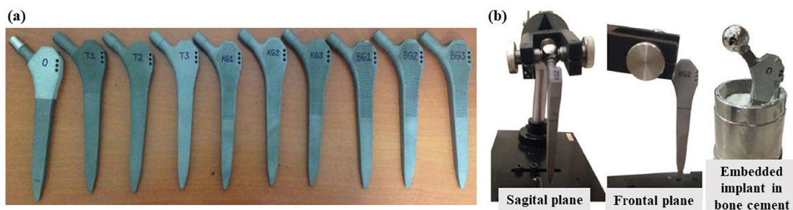
Fig. 28 All specimens produced (a) and experimental setup (b) (images reproduced with permission from reference [246])
