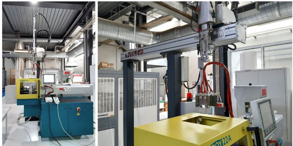
Fig. 4 The BOY 22 A injection molding machine, the PIKO pneumatic robot, and the IR heating system (Laboratory of University of Minho)
