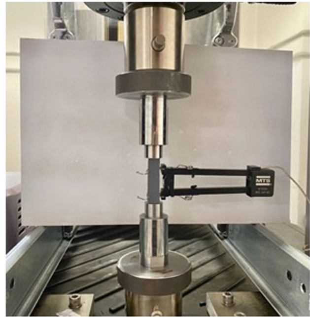
Fig. 4 Picture of the sample during the compression test
