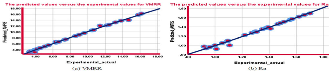
Fig. 10 The predicted values versus the experimental values for a VMRR and b Ra of the ANFIS model
