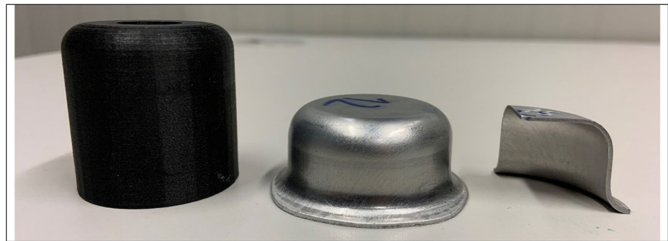
Fig. 4 Polymer punch (left), cup (centre), and cup cross section (right)
