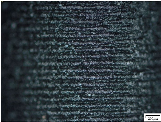
Fig. 23 Side view of a 3D-printed staking post with a layer height of 0.1 mm
