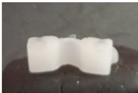
Fig. 12 Example of the deformed part due to difficult ejection of the narrow part
