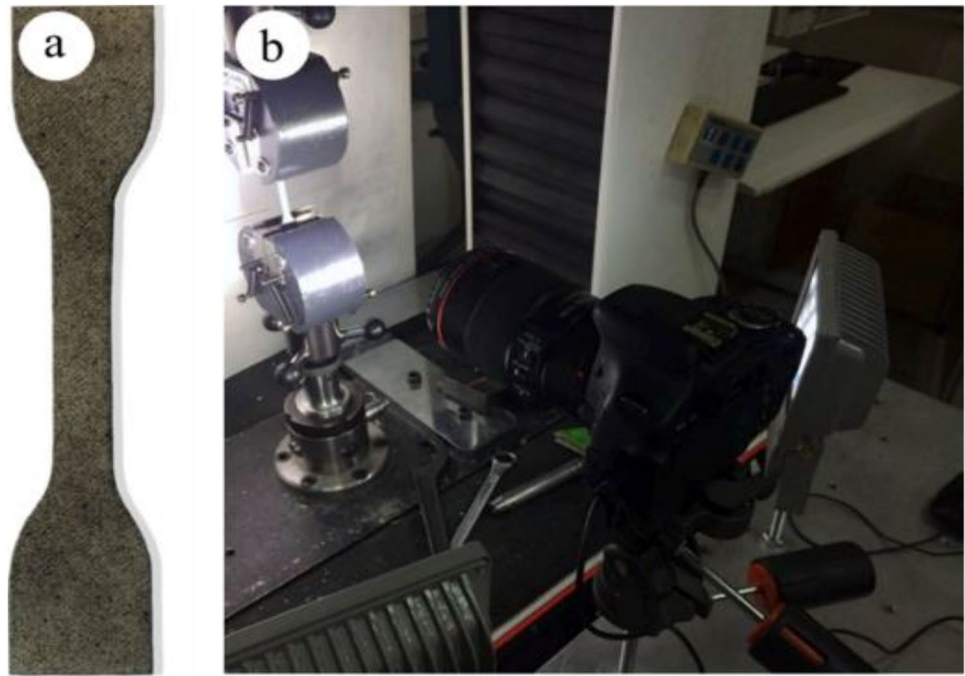
Fig. 2 Characterisation of the mechanical properties of FDM-ABS specimens: (a) Printed tensile specimen and (b) tensile testing configuration [24]
