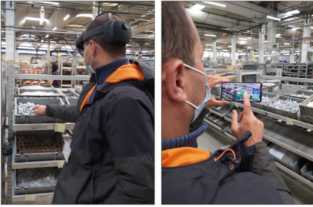
Fig. 8 Participant performing the picking task using the Pervasive AR tool to visualize the kit components location. Left: Using a HMD. Right: Using a HHD
