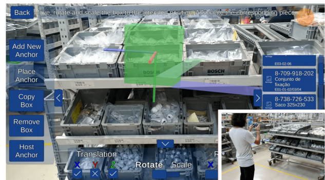
(b) HHD configuration interface. Placing the virtual cube in the correct pose. The association is conveyed using the right-side components list. At the right-bottom corner is possible to observe the user holding the device while performing this action.
