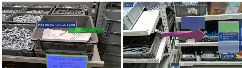
Fig. 9 Examples of an improvement conducted. Directional arrow used to guide operators to the next component to be picked. Left: HMD; Right: HHD
