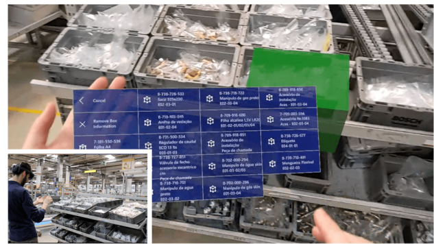
(a) HMD configuration interface. Associating a component to the selected cube. The components list can be accessed through the left hand facing upwards. At the left-bottom corner is possible to observe the user wearing the hardware and performing the corresponding action.
