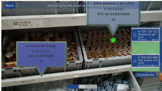
(b) HHD visualization interface. The scroll menu on the right can be used to confirm which components were already picked (highlighted in green) and which were not (in blue).
