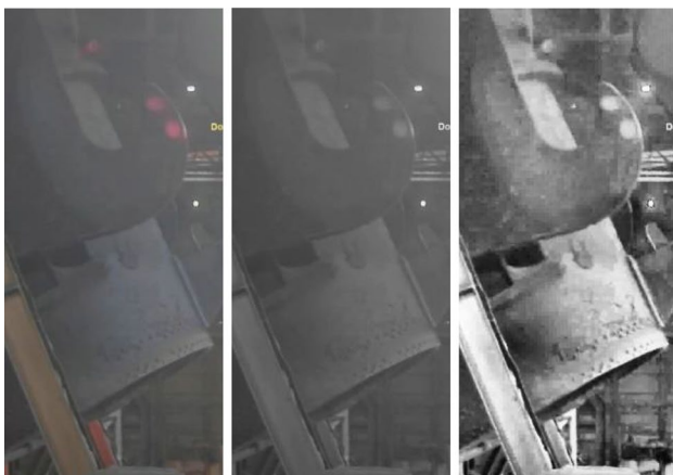
Fig. 8 Ladle edge in original video (left), greyscale video (center) and denoised video (right)
