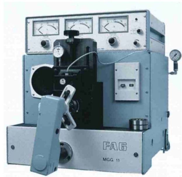
Fig. 8 FAG rolling bearing vibration measurement system equipped a clamp assembly that enables lifting for bearing replacement [33].
