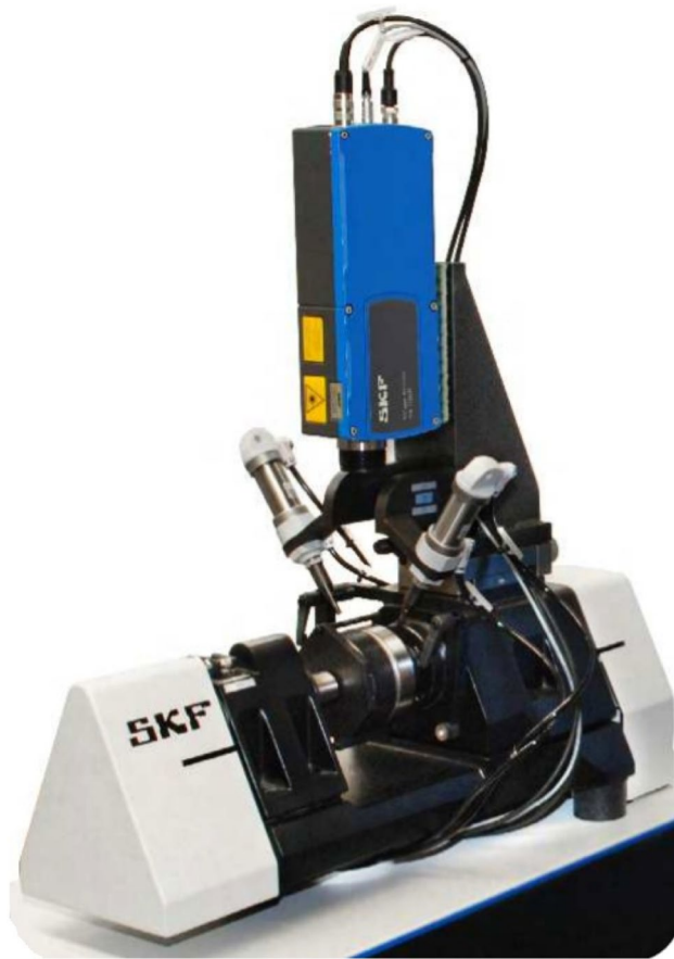
Fig. 14 SKF rolling bearing vibration measurement station head equipped with a laser Doppler vibrometer and containing an additional radial load assembly [23]
