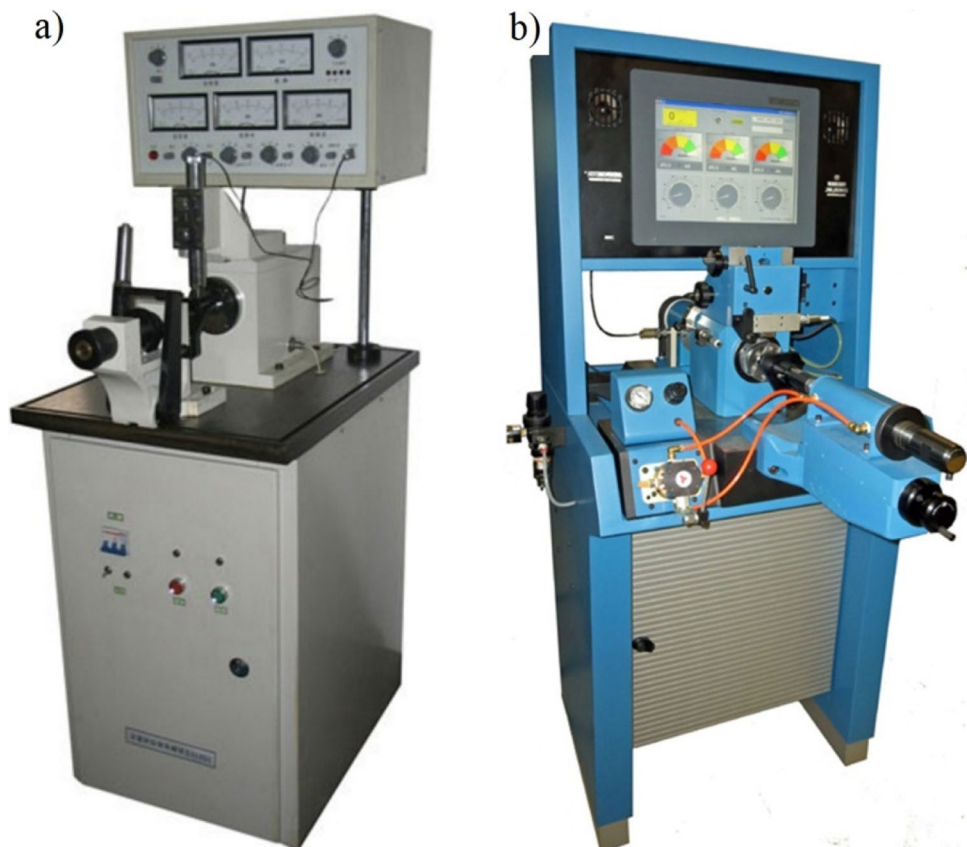
Fig. 10 Various solutions for presenting the results of rolling bearing vibration measurement systems: (a) ZYS station with an analogue panel [24], (b) PDI station with a digital display [27]
