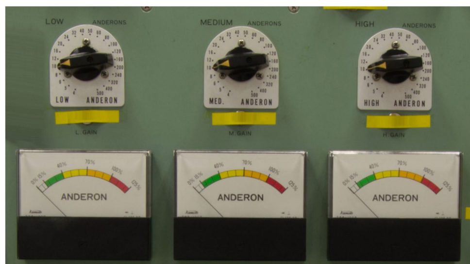
Fig. 11 Panel of the analogue rolling bearing vibration measurement system, indicating the measurement result of the vibration's RMS value in three frequency bands, expressed in Anderons
