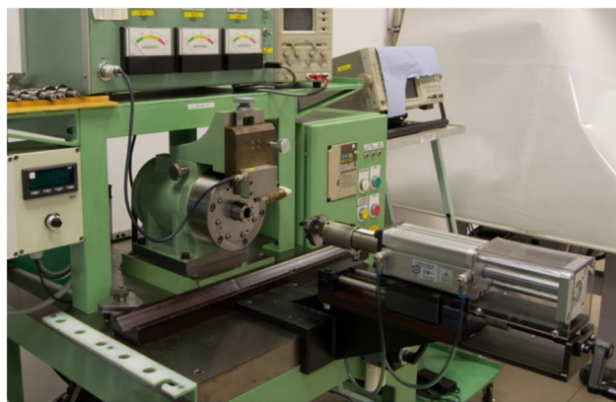
Fig. 3 SUGAWARA test device equipped with an air bearing spindle
