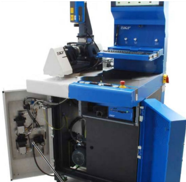
Fig. 5 SKF rolling bearing vibration measurement system [23]
