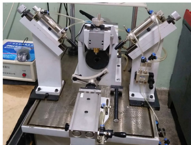
Fig. 13 BTV-6 rolling bearing vibration measurement device containing an additional radial load assembly [15]
