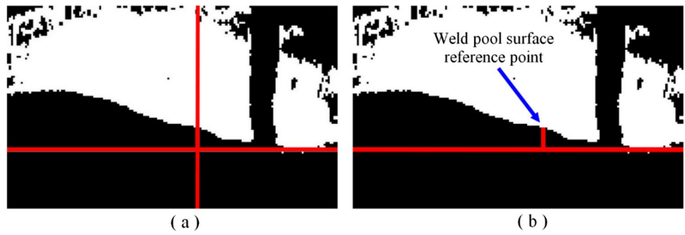
Fig. 3 References for estimating the weld pool oscillation: (a) row and column in the image; (b) point on the weld pool surface
