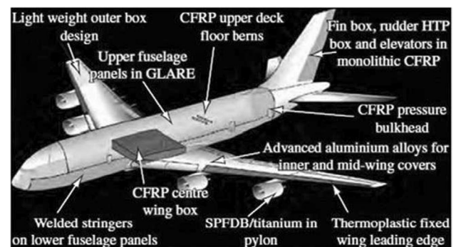
Fig. 1 The functionality of composite assemblies on A380 [5]
