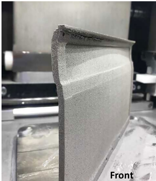
Fig. 5 Example of a build that failed for a thin plate without additional support shown in Fig. 1 and shape data in the top of Fig. 6
