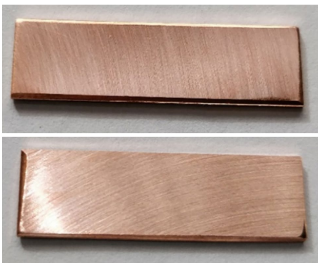
Fig. 9 Sanded copper sheets (500 mesh) with grooves in different directions
