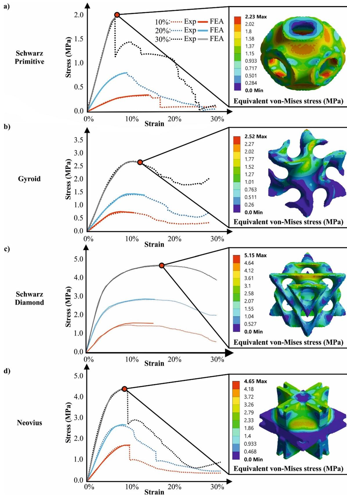
◀Fig. 9 Comparison between the experimental and FEA stress-strain curves, along with the Equivalent von-Mises stresses for: **a** Schwarz Primitive structure, **b** Gyroid structure, **c** Schwarz Diamond structure and **d** Neovius structure
