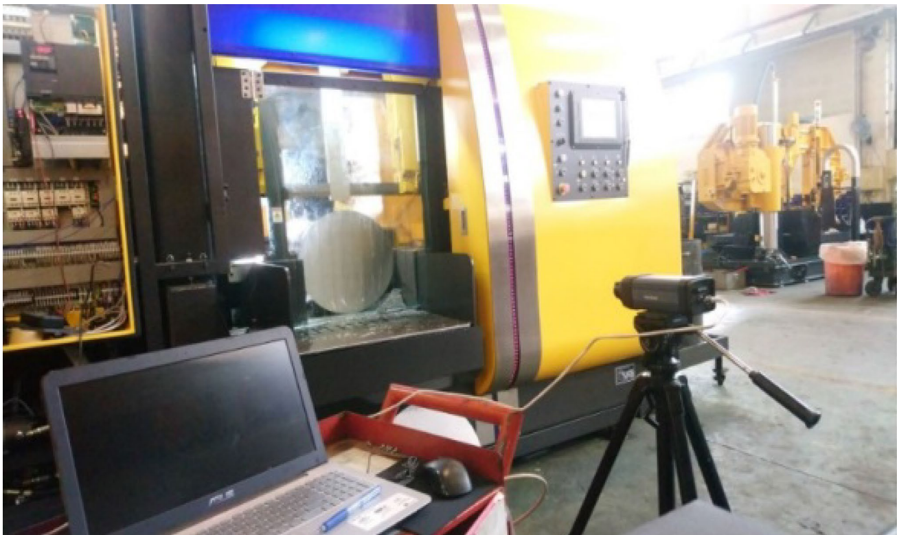
Fig. 1 System setup of sawing process monitoring
