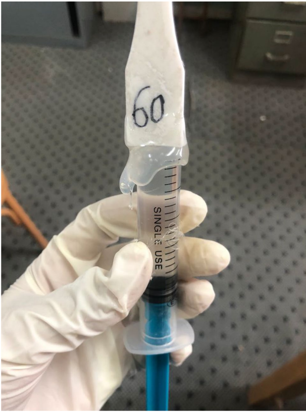
Fig. 4 Injection process of 60% infill tensile specimen
