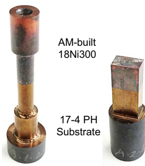
Fig. 4 Pre-machined and heat-treated 18Ni300-17-4 PH samples
