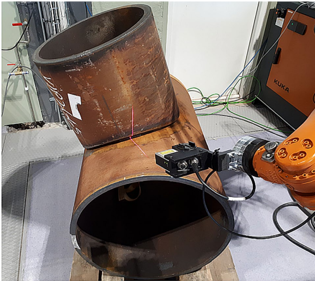
Fig. 7 Experimental setup for testing of the proposed scanning procedure. A commercial laser sensor is mounted on the robot end-effector and is projecting a line towards the weld groove of the tubular T-joint
