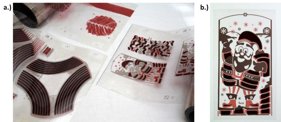
Fig. 10 R2R printed freeform a) OPV films and b) OPV module
