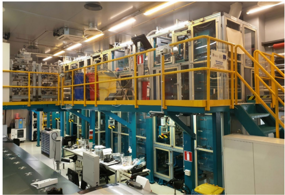
Fig. 8 R2R fabrication of OPV with MAXI pilot-line printing machine using rotary screen printing (RS) for the patterning of ITO electron contact, gravure printing (G) for electron transporting (ETL) and photoactive layer and RS for hole transport layer (HTL) and hole contact layer
