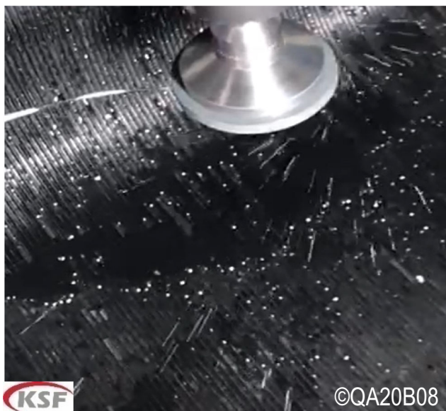
Fig. 8 The coolant is almost tangentially positioned to the grinding wheel and sprayed out of the internal cooling channels of the 3D-printed grinding tool
