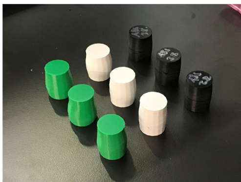
Fig. 4 FDM AM material variation: PETG (green), PLA (white), and ABS (black). Cylindrical specimens are subjected to compression tests to evaluate the mechanical properties of the material
