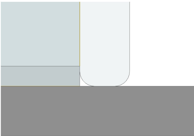
Fig. 10 Side-view of fillet geometry shown in Fig. 8e leading to no intersection for segmentation
