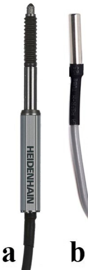
Fig. 11 Displacement (a) and temperature (b) sensors
