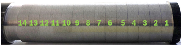
Fig. 1 Numbered workpiece after performing the 14 plunge grinding experiments according to Table 4
