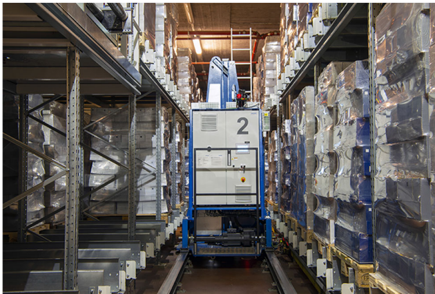
Fig. 1 LTW shuttle system for pallets. Source: LTW Intralogistics GmbH
