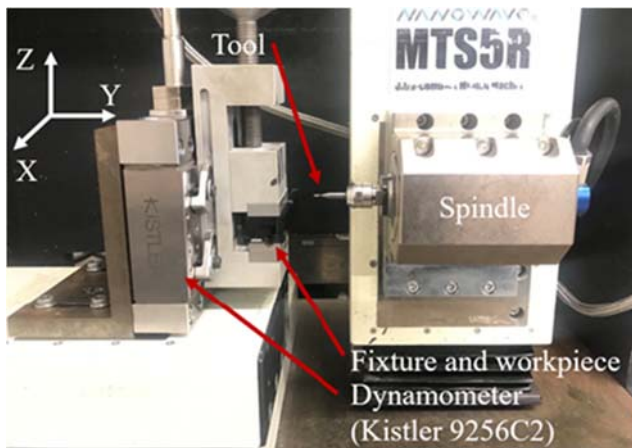
Fig. 4 Machine setup with cutting force dynamometer
