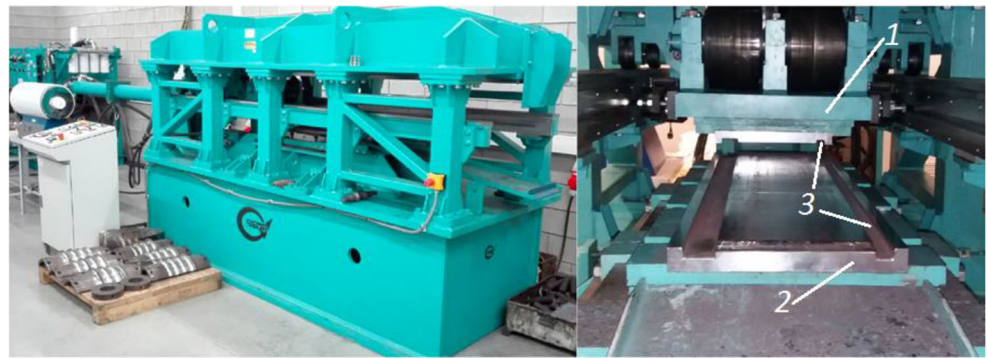
Fig. 2 Test stand (left) and flat tools (right) used in rotary compression in tool cavity test, where 1—upper tool (moving), 2—lower tool (fixed) and 3—tool cavities in which the test-piece is formed
