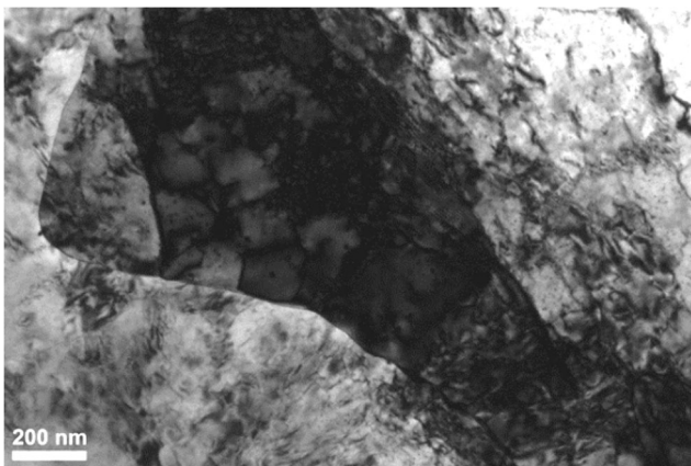
Fig. 8 Typical microstructure (TEM) of Cu1Cr0.1Zr alloy wires extruded by KOBO method at 200 °C
