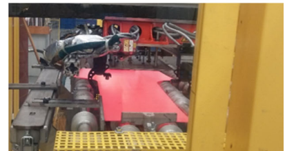
(d) Austenitic blank on roller right after heating.
